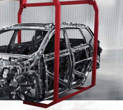
The Tiggo 4 Pro is built on Chery's new six-dimensional beam platform. More than two-thirds of the vehicle's frame and structure is built with high- and ultrahigh strength steel, and the 6-dimensional design gives it unmatched tortional rigidity and crash safety.
